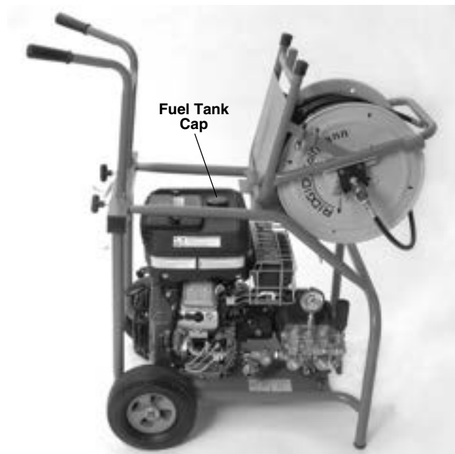
Figure 8 – KJ-3100 Fuel Tank Access
