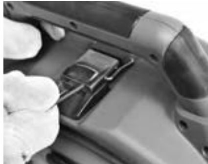
Figure 14 – Open Latch Under Carry Handle (Use Hex Wrench)
