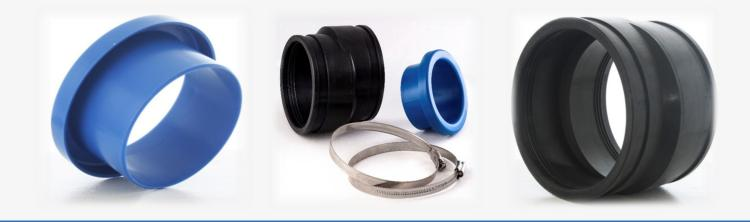
The STEP-Coupling is a secure solution to connect horizontal relined and unlined pipes. The disadvantage of traditional connectors is that there are seams created, increasing the risk of leakage. In addition it is difficult to achieve the desired results using traditional solutions. With Repipers STEP-Coupling watertight connections are created without seams or gaps.
